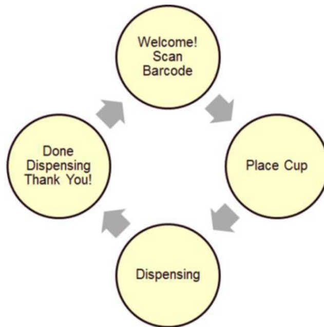
FIGURE 38: LCD STATE DIAGRAM
